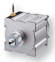
Encoders with a prefixed draw-wire sensor (0.25 to 40 m long) are the best choice for direct length measurements. Thanks to the excellent repeatability rating of 0.05 mm, they solve position control tasks with the utmost precision in applications which, up to now, could only be handled by complex equipment.
