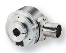
Absolute singleturn encoders detect any angle within a full revolution of 360°. With absolute encoders, each incremental angle is assigned a code pattern. This allows the position to be detected at any time, even after a power failure, without having to initialize a reference run. Absolute encoders detect angles, positions and inclinations precisely – tasks, that are typically found in robotics, positioning and process technology.
